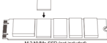
(Optional) Remove the protective films and then paste the small piece thermal pads to the chip(s) that is thinner than others. You want to make sure all chips are at the same height for best conductive heat transfer.
